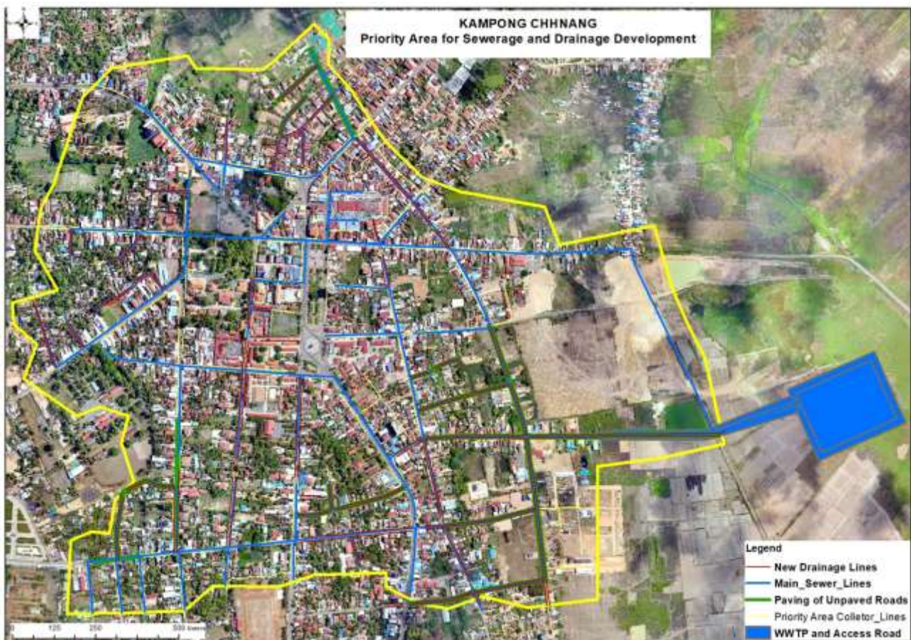
Figure 2: Layout of the Sewerage and Drainage Systems
