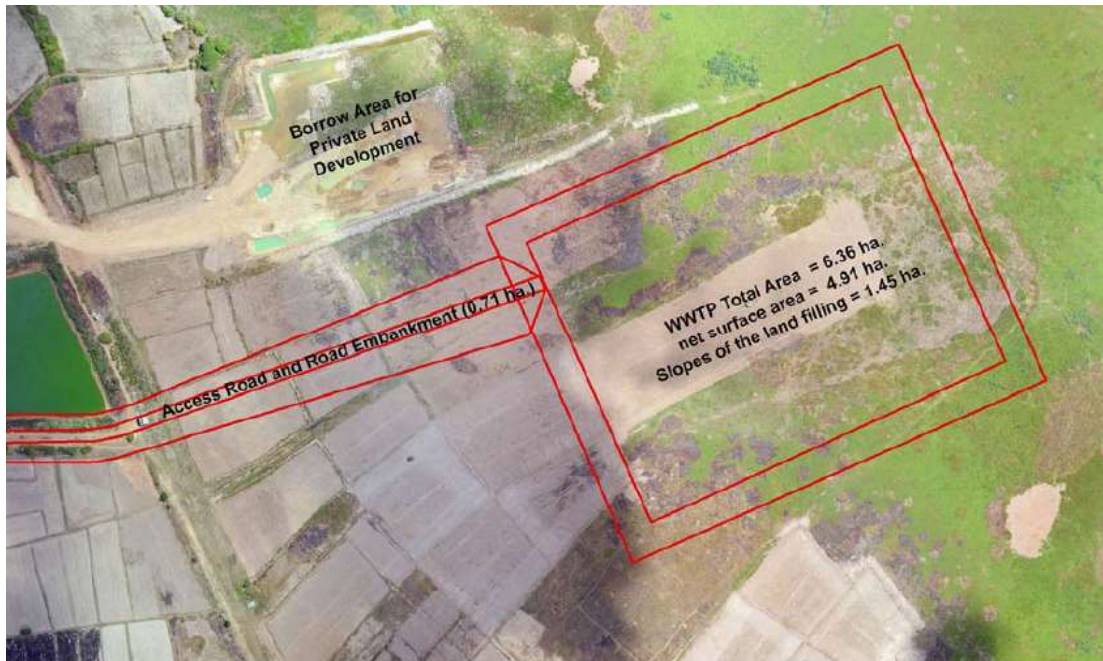
Figure 5 WWTP site location and access road
