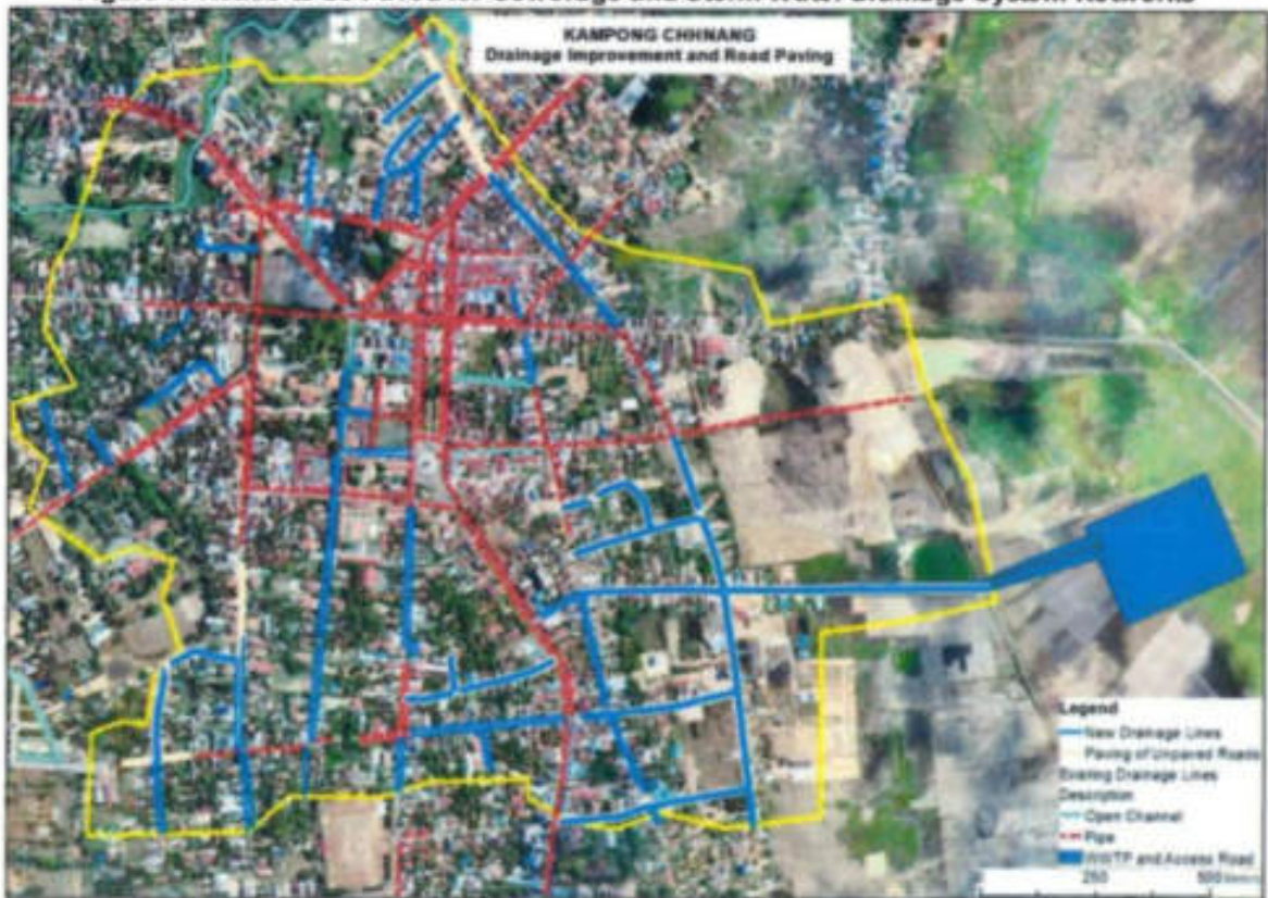
Figure 7: Roads to be Paved for Sewerage and Storm Water Drainage System Networks
