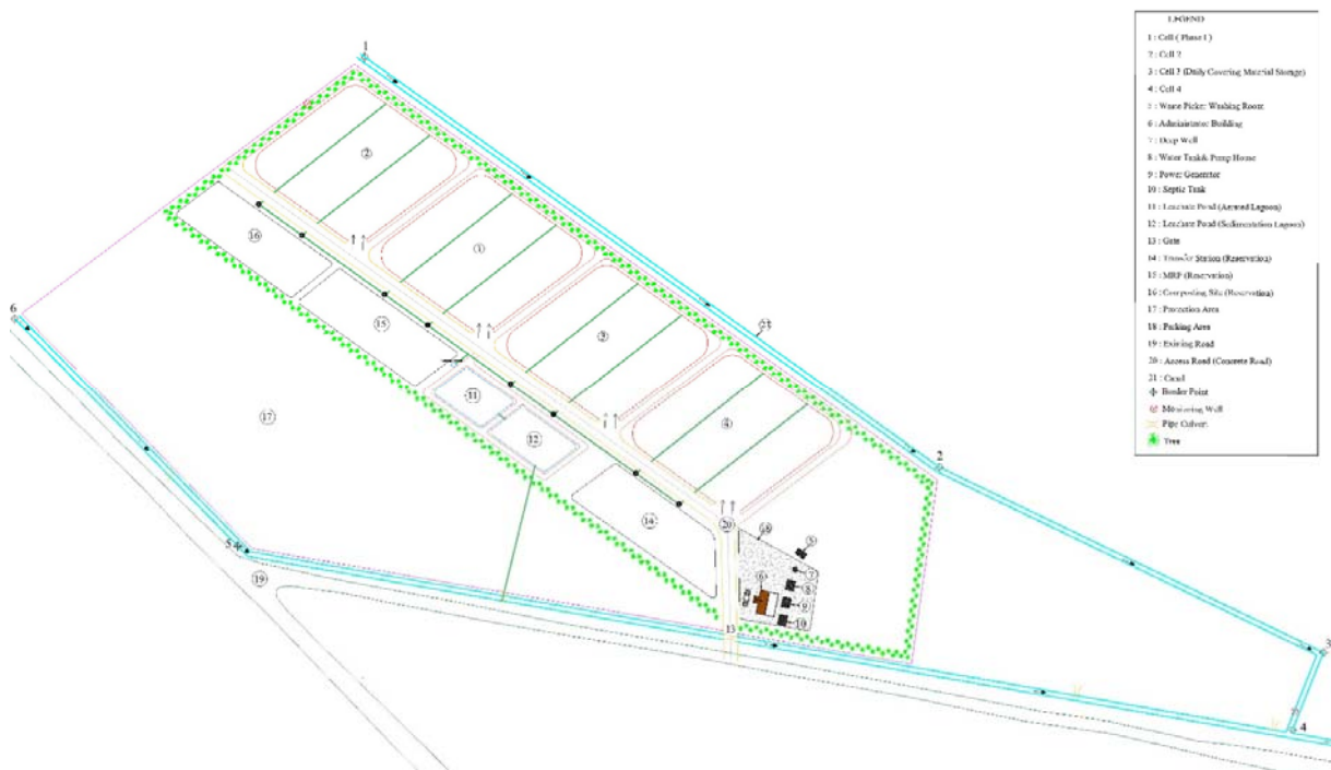
5-2 Layout Kampong Chhnang Controlled Landfill
