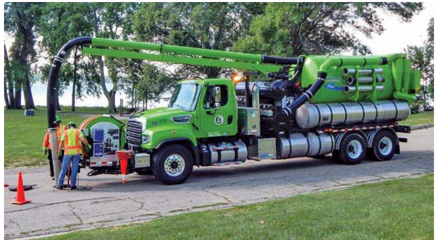
Proposed Jet-Vac combo truck. The combination jet/vac process consists of a hose and nozzle that is propelled forward in the sanitary sewer line by high water pressure. Debris, slurries, sludges that is loosened by the water pressure is forced to the manhole from where it is hydraulically sucked out by a vacuum pump
