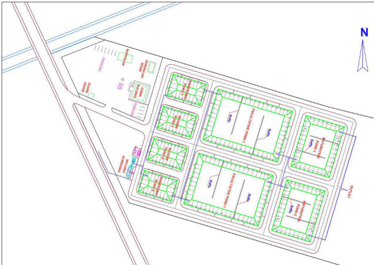
Figure 5. Typical STP Layout
