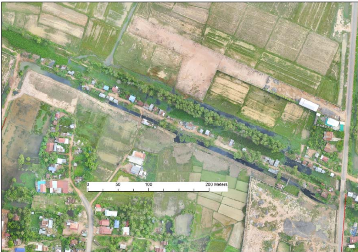
Photo 1: Pools of stagnant sewage between the two outfall points of the Pursat Drainage system
