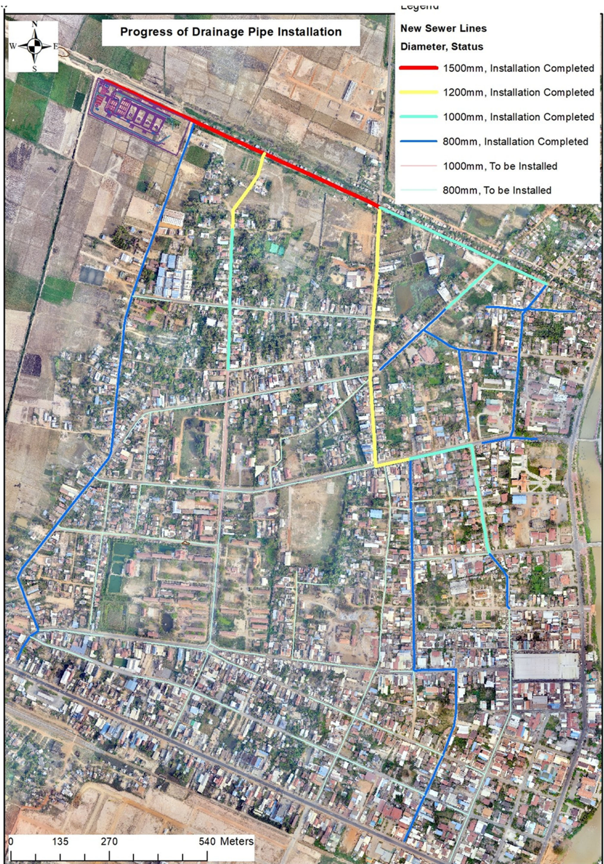
Figure 4-4: Progress of the installation of new drainage pipelines
