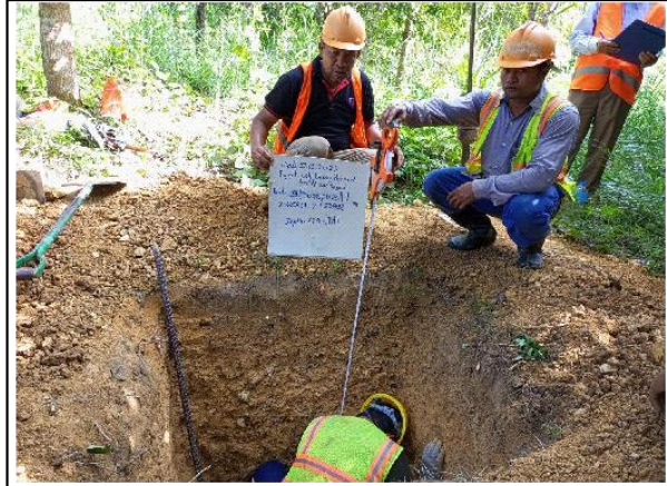
Excavated pit, 1.5 m deep and Carry out Dynamic Cone Penetrometer text
