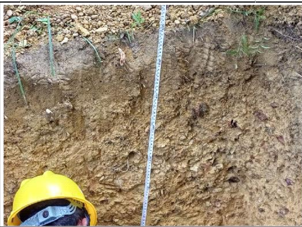
Excavated pit, 1.5 m deep and Carry out Dynamic Cone Penetrometer text
