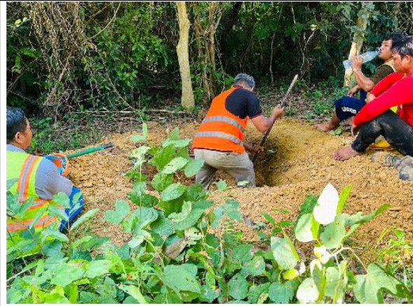
Excavated pit, 1.5 m deep and Carry out Dynamic Cone Penetrometer text
