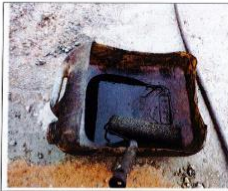
e. Used oil applied to paint forms for precast U-drain
