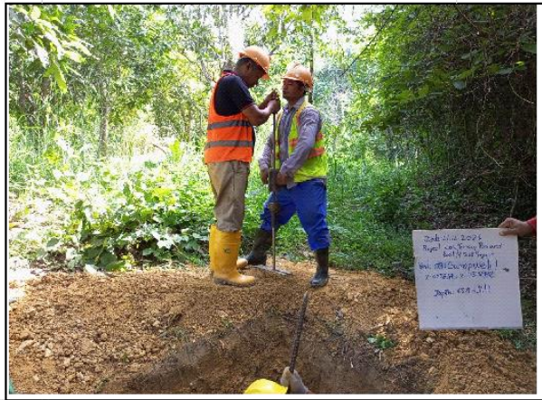
Excavated pit, 1.5 m deep and Carry out Dynamic Cone Penetrometer text
