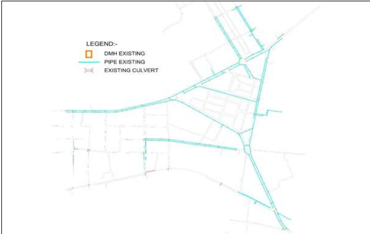
Figure 2: Existing Drainage System
