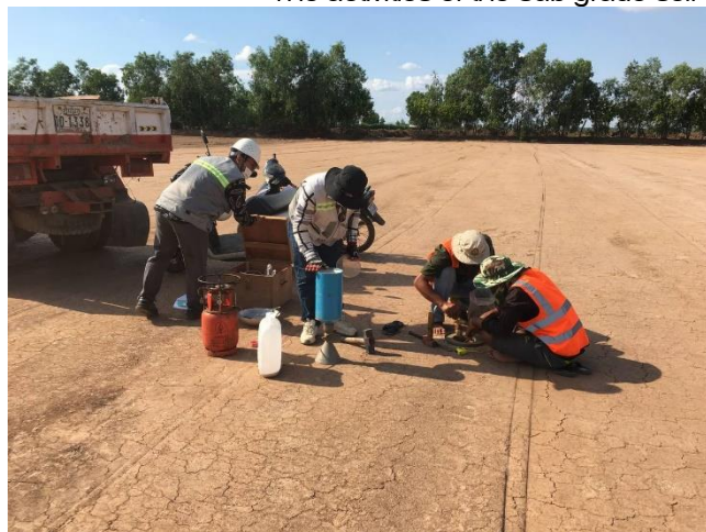
The activities of the sub grade soil test ( FDT ) and pipe pre-casting
