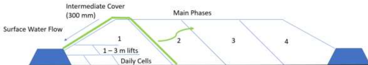
Figure 13: Battambang Landfill design approach
